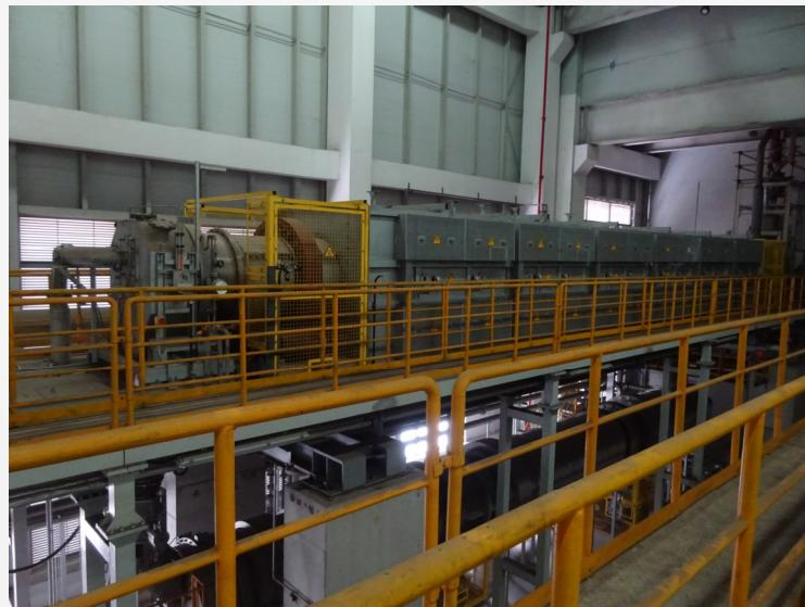
DRA 16/100-E-85 with separate Air Cooling Pipe CP12/120-A, increased O2-Atmosphere
